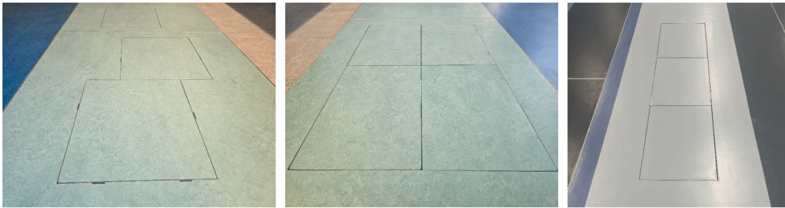
Fig. 1. Examples of the arrangement of force plates depending on the type of movement being measured, as well as the size and stride length of the patients. LEFT: Three staggered force plates, the first two intended for children (shorter stride length), plates 2 and 3 for adults. CENTER: Parallel arrangement, specifically for jumps or sit-to-stand analyses. RIGHT: Arrangement in a row, for adults, sit-to-stand analyses are also possible.
